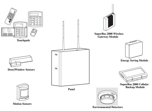
Figure 1. Security System Components
